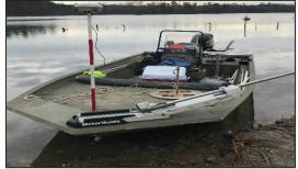
POS/MV Wavemaster: All Arc Surveying vessels are equipped with a POS/MV Wavemaster, a tightly-coupled system using Applanix' unique approach to Inertially-Aided Real-Time Kinematic technology. The user-friendly, turnkey system provides accurate attitude, heading, heave, position, and velocity data, representing the latest in state-of-the-art inertial/GPS technology. The system maintains positioning accuracy
